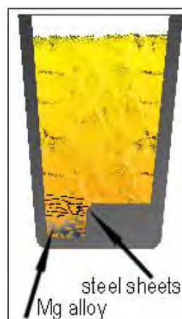
Figure 2.23: The sandwich method for nodularisation [237, HUT, 2003]
