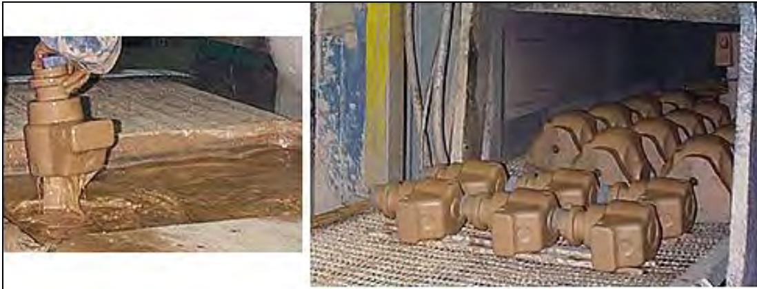
Figure 2.35: Dip-coating with water-based coatings, followed by drying in a hot-air furnace [237, HUT, 2003]
