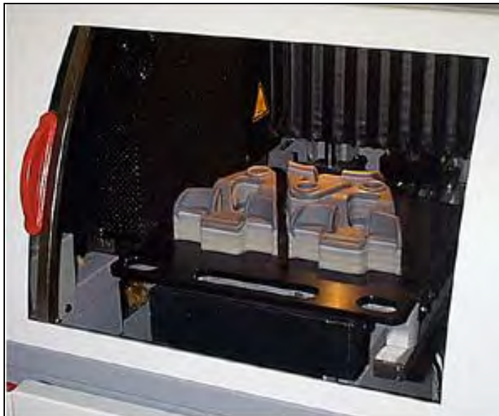
Figure 2.6: Thermopolymer (wax) patterns in an RP machine [237, HUT, 2003]
