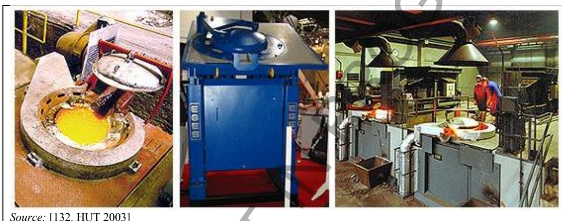
Figure 2.18: Coreless induction furnaces
