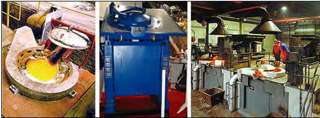
Figure 2.14: Coreless induction furnaces [237, HUT, 2003]
