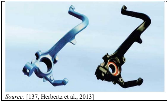
Figure 1.24: Forging before (left) and after mechanical processing (right)
