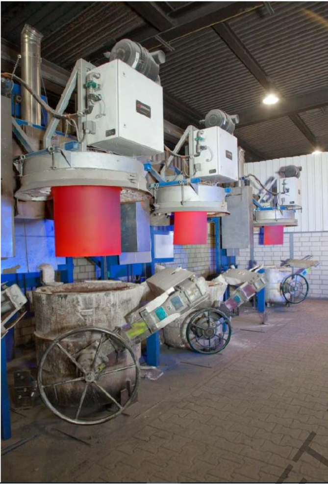
Figure 3.6: Ladle preheating using porous burners
