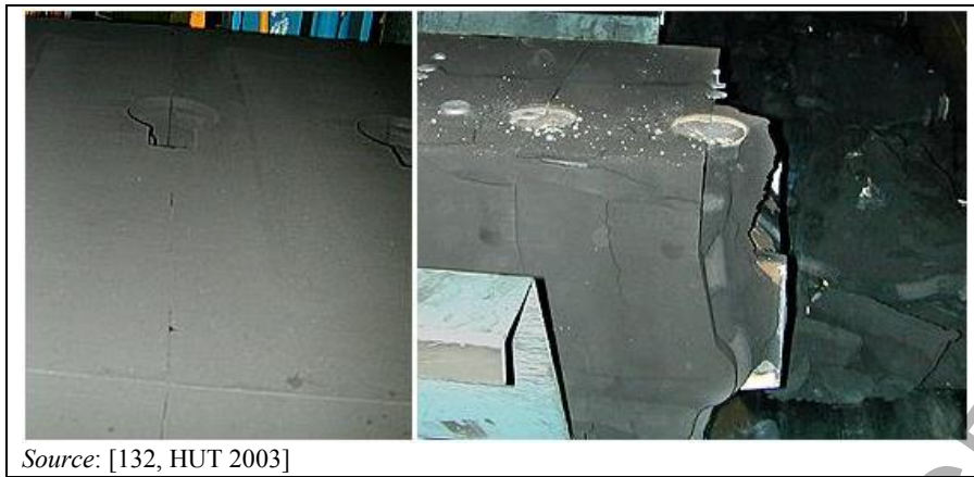
Figure 2.47: Shake-out at the end of an automated moulding line
