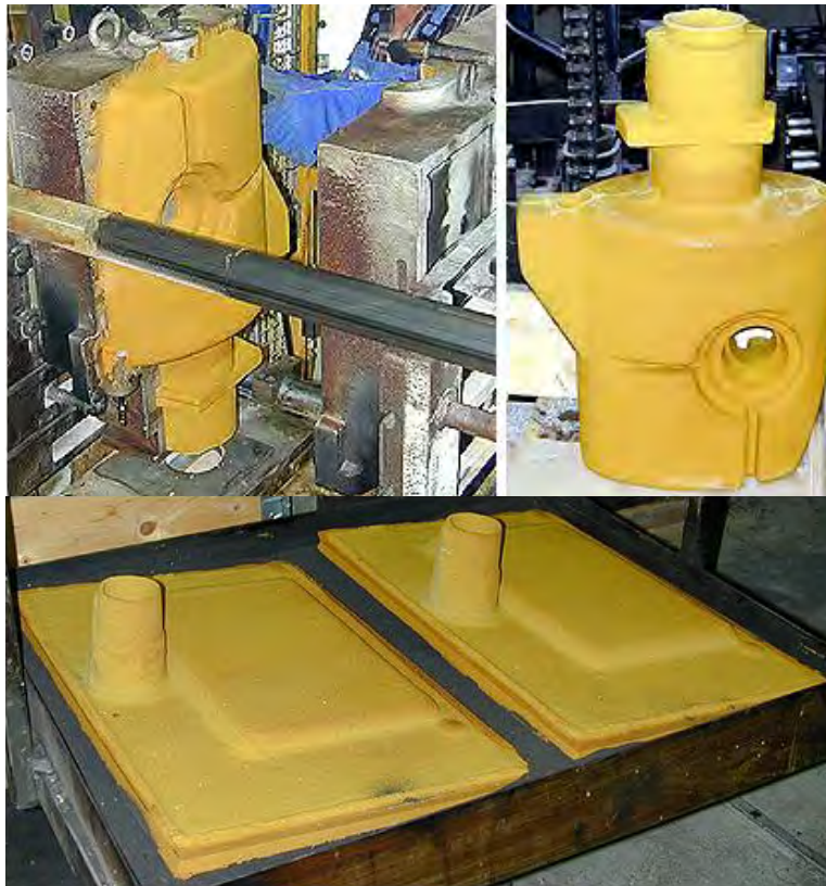
Figure 2.33: Croning cores (top) and moulds (bottom) [237, HUT, 2003]
